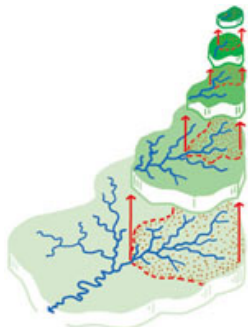
Figure 1: Left: Schematic of precipitation in a watershed flowing to the outlet point (Credit: The COMET Program). Right: A schematic of how watersheds are nested and watershed size varies depending on the basin outlet selected (right, credit: Marsh, 1998, p. 170)
