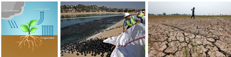
Figure 1: Schematic of ET (left), shade balls dumped into a reservoir to mitigate evaporation (middle) and a dried agricultural field due to excessive evaporation (right).
