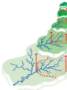
Figure 19: A schematic of a watershed and its divide (left, credit: Alice Ferguson Foundation ). A schematic of how watersheds are nested (right, credit: Marsh, 1998, p. 170)
